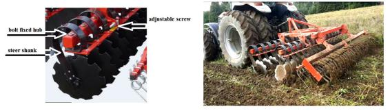
Fig. 1. Experimental aggregate compact disc harrow "KBT-4"
